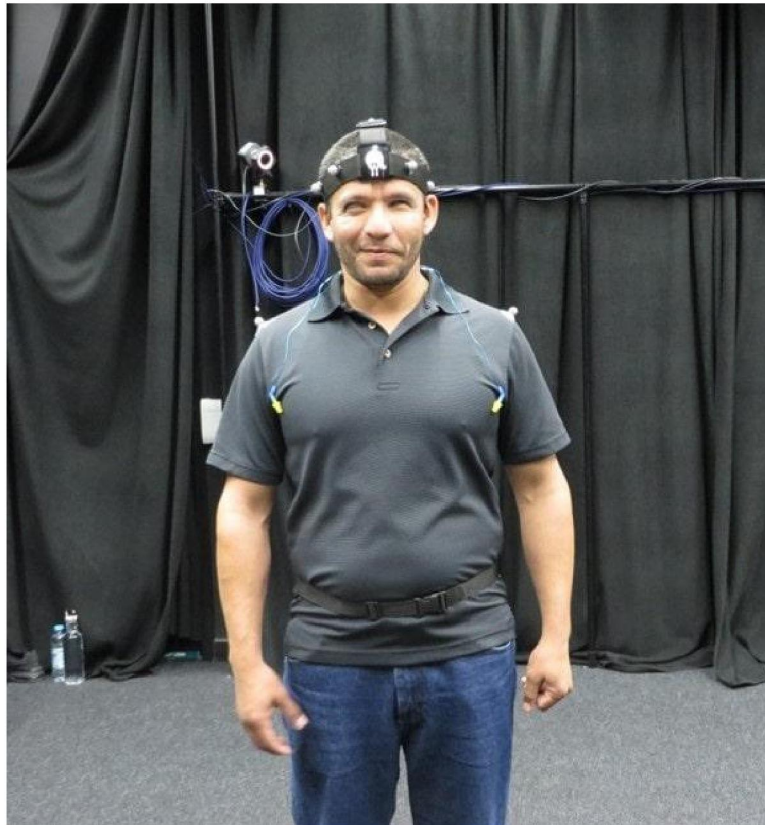
Figure 4. Photograph of the experimental set up used to record head movements that echolocators make during echolocation. Juan Ruiz is wearing reflective markers on his head. Special cameras track these markers, and we can use these data to reconstruct the movements of the head. Credit: Nina Ruiz
