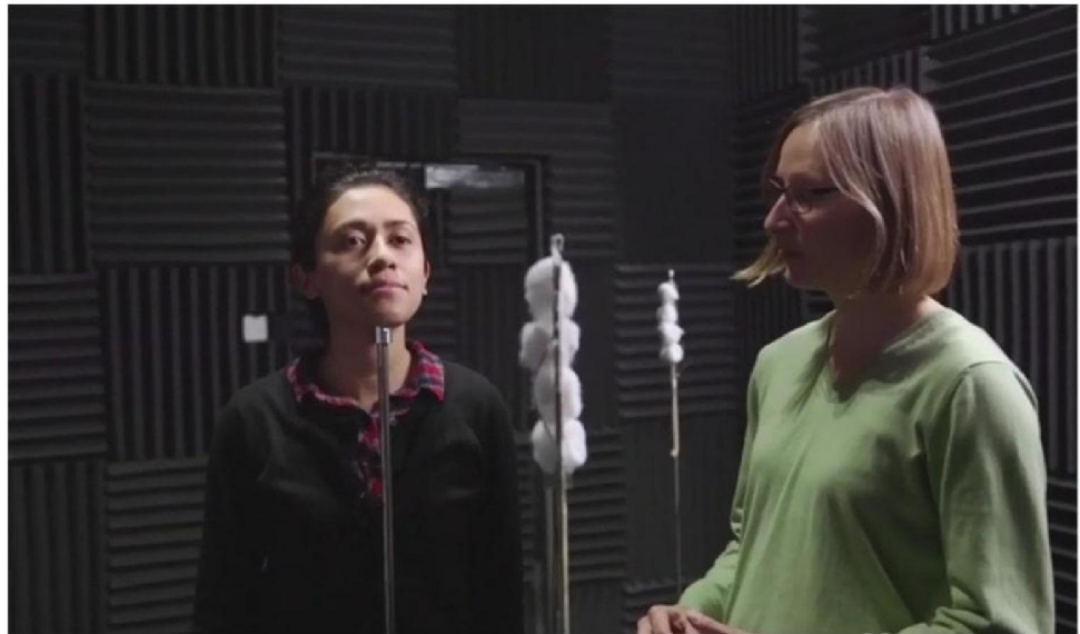
Figure 2. Photograph of the setup used to make recordings of echolocation mouth clicks. Recordings are made in rooms that are insulated against outside noise, and the walls, ceilings and floors of which are covered in special foam. Thin metal poles covered with cotton wool are used to hold microphones, and another metal pole is provided for positional guidance for the person making mouth clicks. During recordings only the person making clicks is inside the room. The experimenter controls the equipment from outside the room. Credit: Lore Thaler
